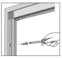
12. Install the door post with magnet. Align the top rail and the stop post in the center and fix it with tapping screws.
