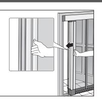
Make sure to hold the central part of the sliding bar to open & close the unit. Push it onto the door post. It easily closes as the magnet is slotted in the door post. Note: If you try to operate the sliding bar at the extreme edges, it may make the operation unsmooth.
