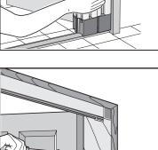
②At this point, the anchor plates are only temporarily attached to the door installation frame with its both-sides-adhesive-tape so they must be fixed with tapping screws. Note: Don't tighten the screws too far as this may break the anchor plates. So you should tighten the screws by hand.
