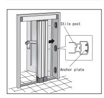
(9)Keeping the bottom of the screen door unit in contact with the bottom rail, align the stile post with the projections of the anchor plate and press it firmly to fit the screen door unit in place.
