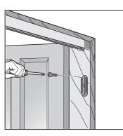
anchor plate. ⑤Fix the anchor plates with tapping screws. Note: Don't screw in the tapping screws too tightly. The anchor plate may get broken. Don't use the electric screw driver.
